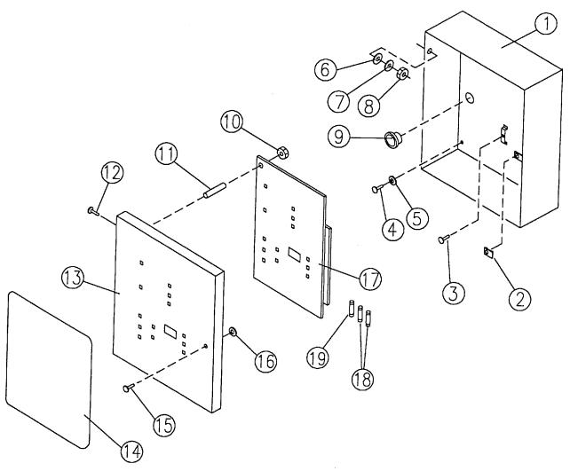
CONTROL BOX ASSEMBLY 150 Lb. Dryer with Reversing
