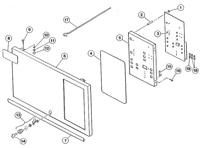
CONTROL PANEL & ACCESS DOOR ASSEMBLY 50/75 Lb. Dryers Reversing/Non-Reversing
